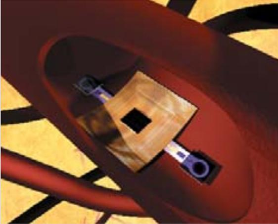
Artist's conception of a pressure/flow-sensing device embedded in the wall of an artery.
